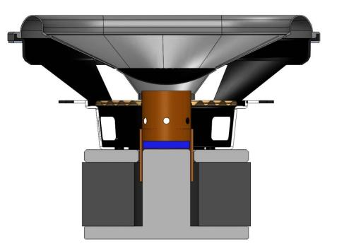
Figure 4 - RCC 4" x 6" Woofer Cross-Section
