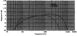
Frequency response of the 2118H/J in a closed box of 14 L (0.5 ft<sup>3</sup>) internal volume. Measured response of a typical production unit, including all peaks and dips, does not deviate more than 2 dB from the above curve. The dashed curve represents the response with a 30 cm<sup>2</sup>(5 in<sup>2</sup>) port, 8 cm (3 in) long, tuning the enclosure to 70 Hz.
