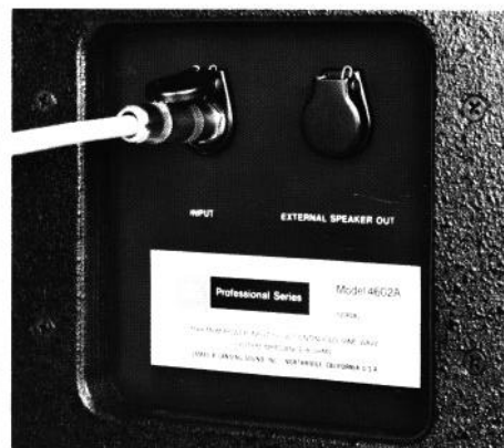
Recessed Input Connectors. Input and external output phone jacks are protected by spring-loaded covers to maintain acoustic integrity of enclosure. High current capacity telephone-type jacks provide positive high power connection.
