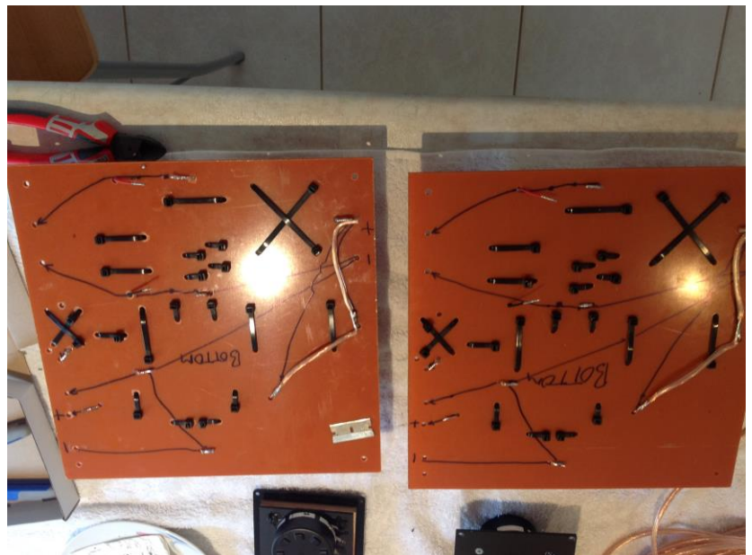
Figure 8: Wire positions marked - Start soldering
