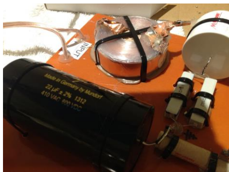
Figure 9: Use hot glue to secure wires and components
