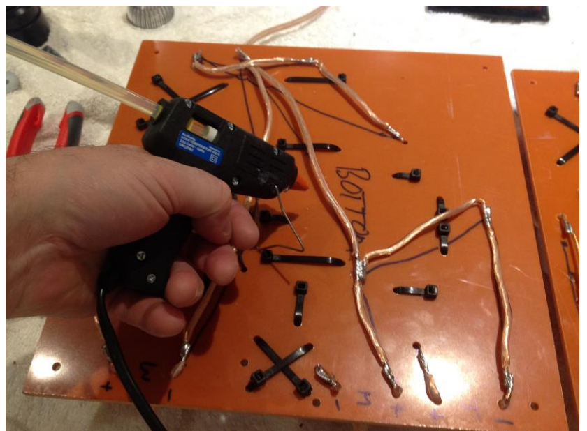
Figure 9: Use hot glue to secure wires and components
