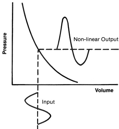
greater distortion as the wave propagates down the horn. The more rapidly the horn flares outward, the lower the pressures become, and the lower the distortion will be.
