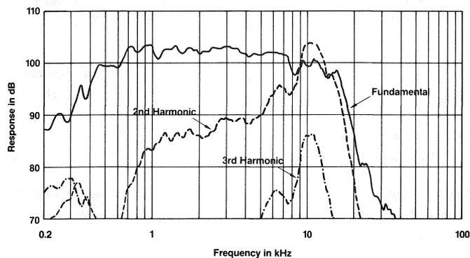
F. Distortion in high frequency drivers is largely a function of acoustical output, not electrical input. The advantage of a large driver over a smaller one is reduced harmonic distortion for the same acoustical output.
