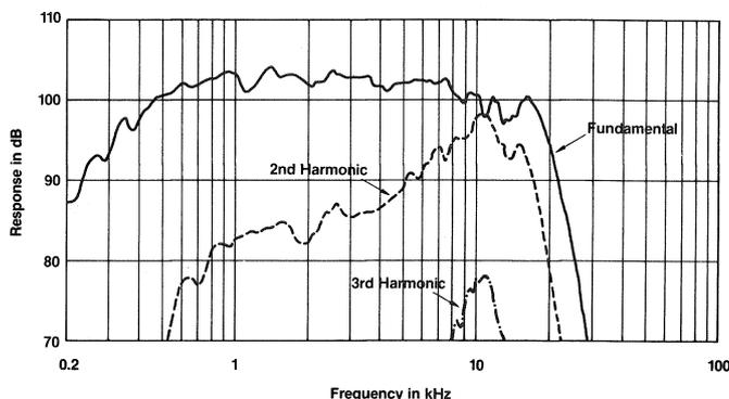
The drive levels used in these measurements are typical of horn/driver combinations which have been equalized for flat power response. Second harmonic components rise fairly gradually and are apparent throughout the midband. For a given intensity, second harmonic distortion doubles with each doubling of driving frequency.
