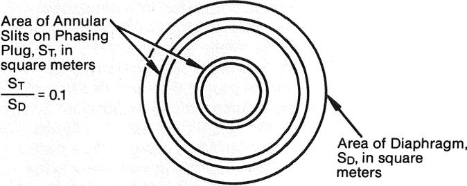
B: End View of Phasing Plug, Diaphragm Removed
