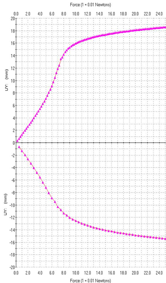
Figure 2 - Suspension Linearity
