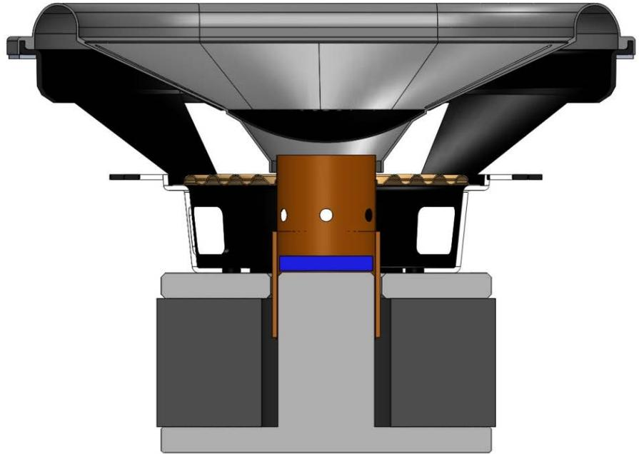
Figure 4 - RCC 4" x 6" Woofer Cross-Section
