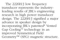
To increase power handling while reducing power compression, JBL engineers created a unique, direct voice coil-to-air heat dissipation method called Vented Gap Cooling. This process pumps air through the magnetic gap and directly over and around the voice coil to provide immediate heat transfer and reduction in operating temperature – a direct improvement in power compression.
