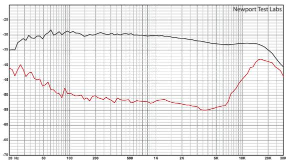
Graph 2. Frequency response (black trace) and channel separation (red trace). [Audio-Technica AT95X]
