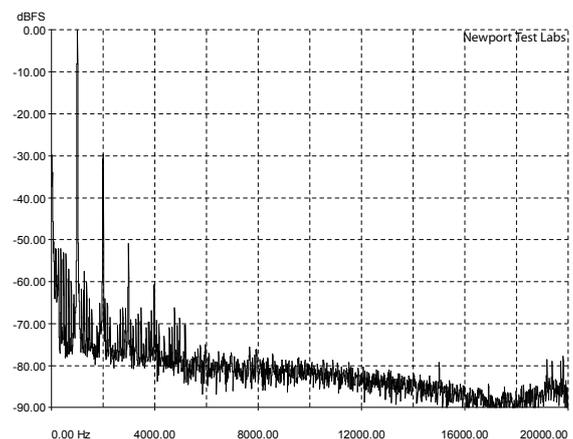
Graph 3. THD at 1kHz, at 3.54cm/second. [Audio-Technica AT-95X Moving-Magnet]
