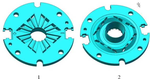
Figure 4: The front phasing plug. 1 – The side of the phasing plug adjacent to the rear phasing plug. 2 – The side of the diaphragm adjacent to the diaphragm.
