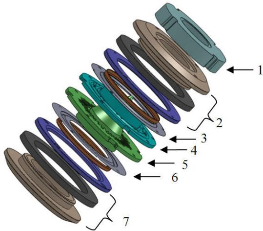
Figure 5: Exploded view of the JBL dual driver D2430K based on 3" voice coil and having 1.5" exit. 1 – front adapter, 2 – front motor, 3 – front diaphragm assembly, 4 - front phasing plug, 5 – rear phasing plug, 6 – rear diaphragm assembly, 7 – rear motor
