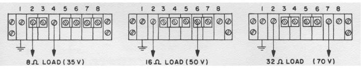
**Speaker Matching:** Use the output tap which most nearly equals the total speaker impedance. If the load impedance falls between two output tap values, use the lower tap.
