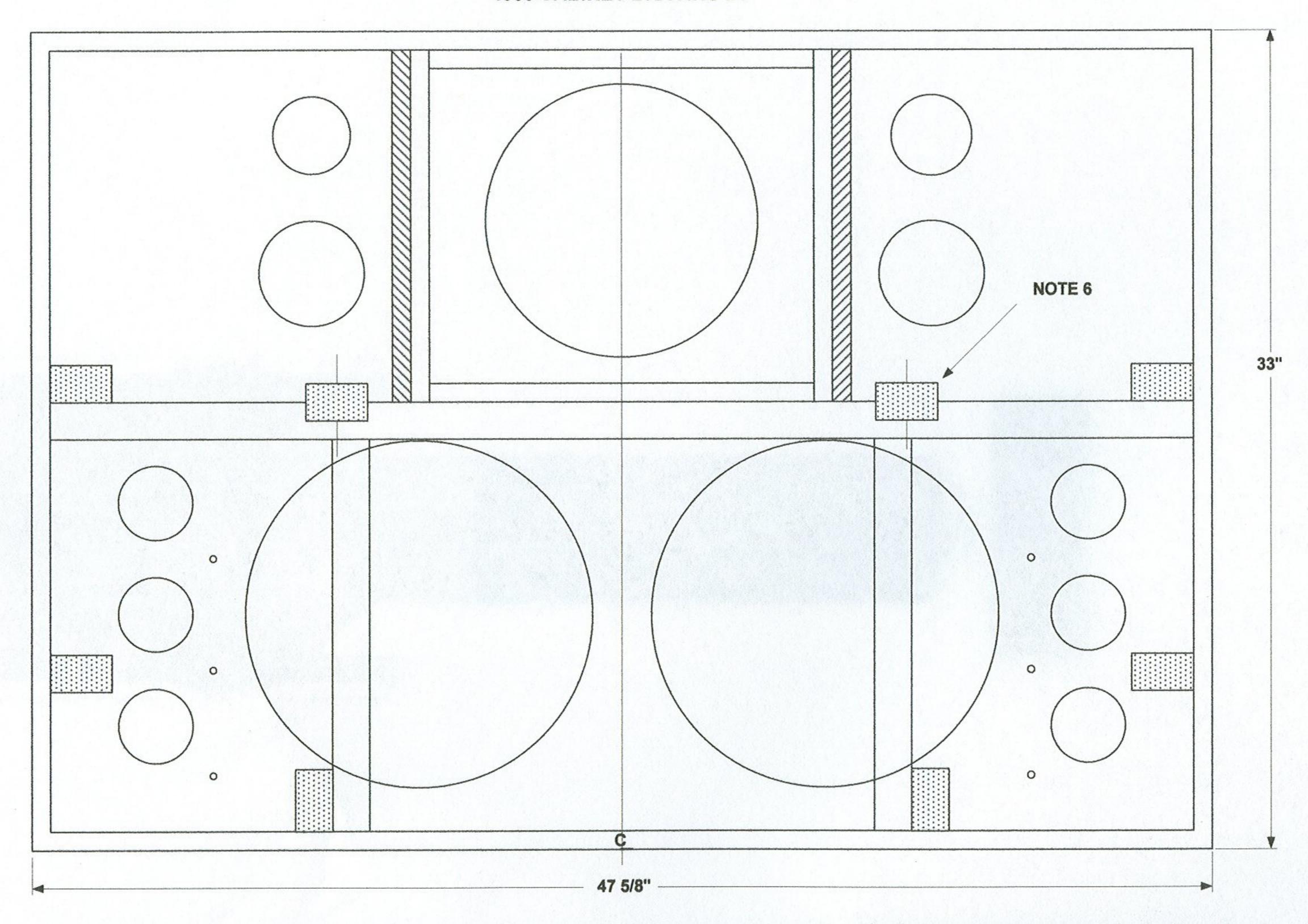
ALL INTERNAL CABINET BRACES ARE 1 ½" x 2 ½". FACTORY CABINETS USED INEXPENSIVE PINE. FIR OR POPLAR WOULD BE BETTER CHOICES. ALL BRACES ARE GLUED AND SCREWED TO THEIR RESPECTIVE PANELS PRIOR TO CABINET ASSEMBLY. ON SOME CABINETS, THAT APPEAR TO BE MID TO LATE PRODUCTION (4350'S), THE BACK BRACES WERE GLUED AND NAILED FROM THE OUTSIDE. THE NAIL HEADS ARE VISIBLE THROUGH THE BLACK PAINT ON THE CABINET BACK.
