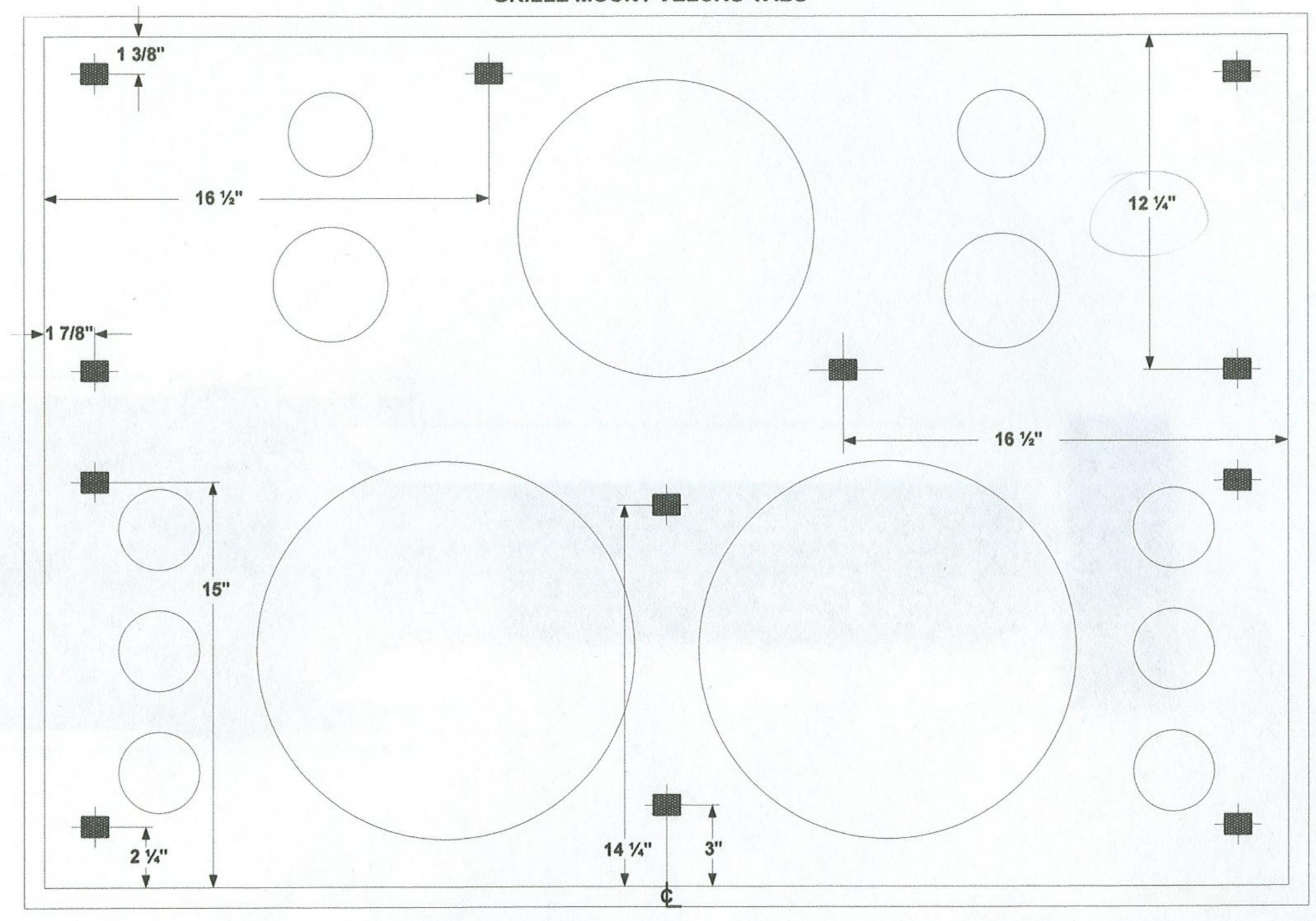
VELCRO TABS ARE ¾" HIGH X 1" WIDE WITH SELF ADHESIVE PEEL AND STICK BACKING. EACH TAB IS STAPLED IN TWO PLACES WITH ½" CROWN WIRE STAPLES.
